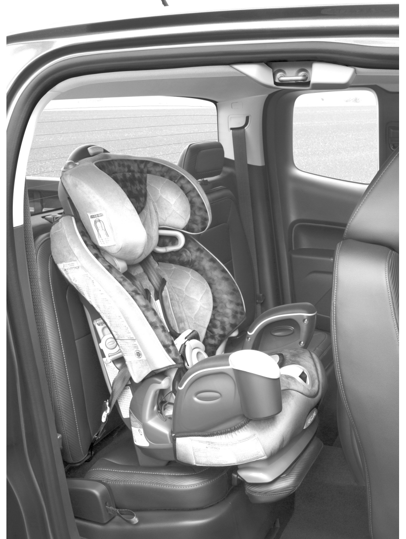
The 2015 GMC Canyon with segment safety firsts including a patent-pending child safety feature. Utilizing the rear jump seat headrest on the passenger side of the extended cab Canyon, the base of the jump seat can be extended to meet NHTSA's recommendation by removing the headrest and inserting it horizontally. PHOTO © GENERAL MOTORS.
